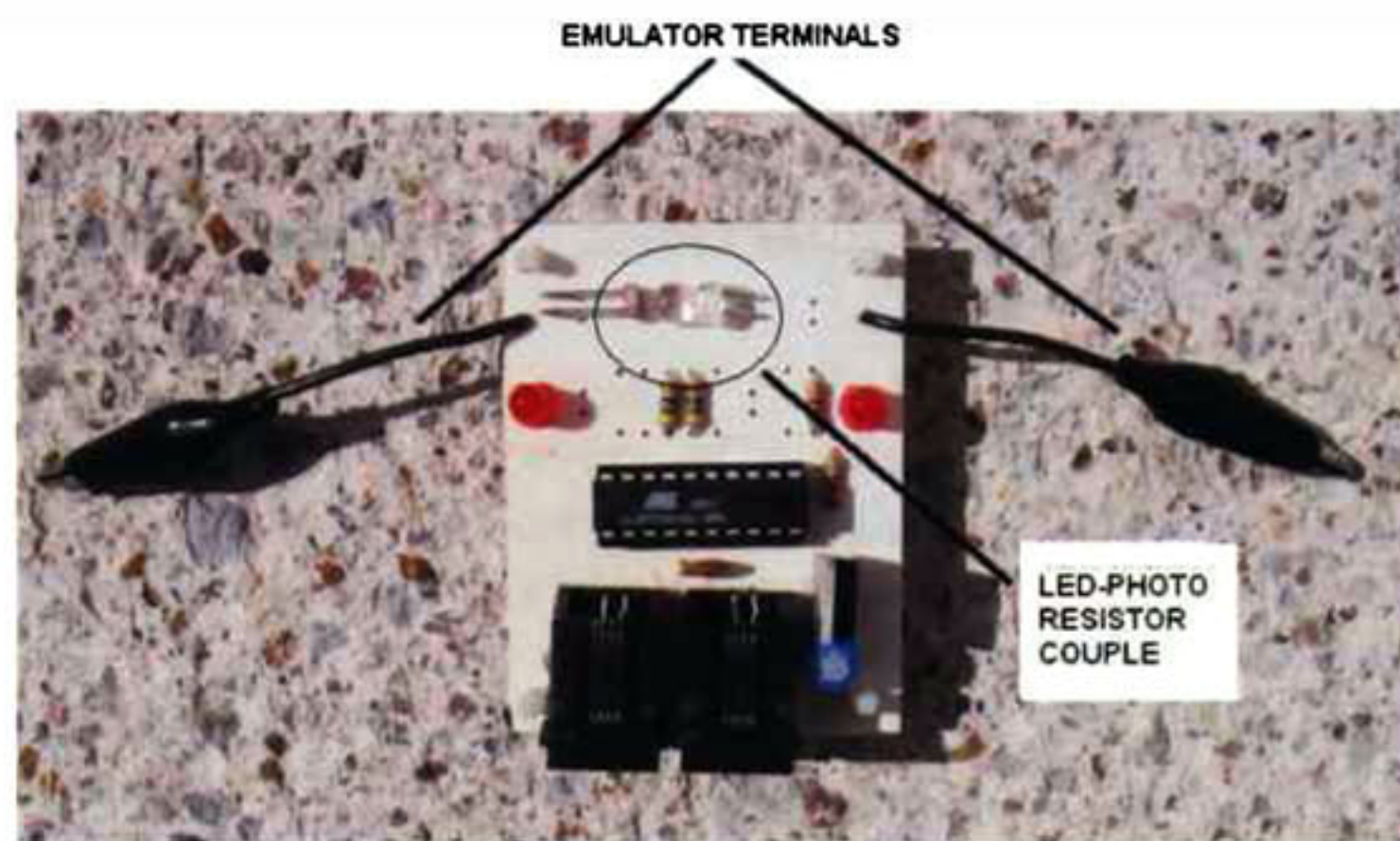
Figure 9, Photograph of the Non-linear emulator device, terminals and the photo-resistor couple are pointed, it also can be seen the microcontroller integrated circuit.
