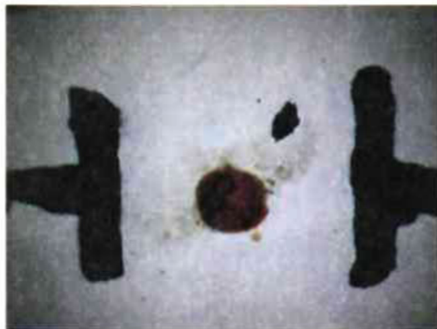
Figure 3. 14 Device used to test Ions displacement and depletion on paper-based optical devices, brown spot at the center is \text{FeCl}_3 to visualize Ion transport inside the device, black spot up-right is to indicate the positive side of the electric field applied through the electrodes at both sides.
