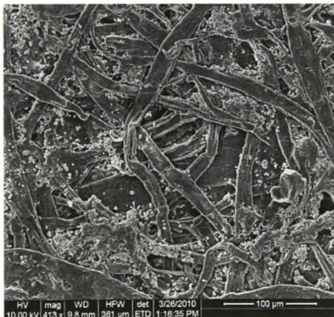
Figure 4. 1 Cellulose fibers from a paper sensor.
