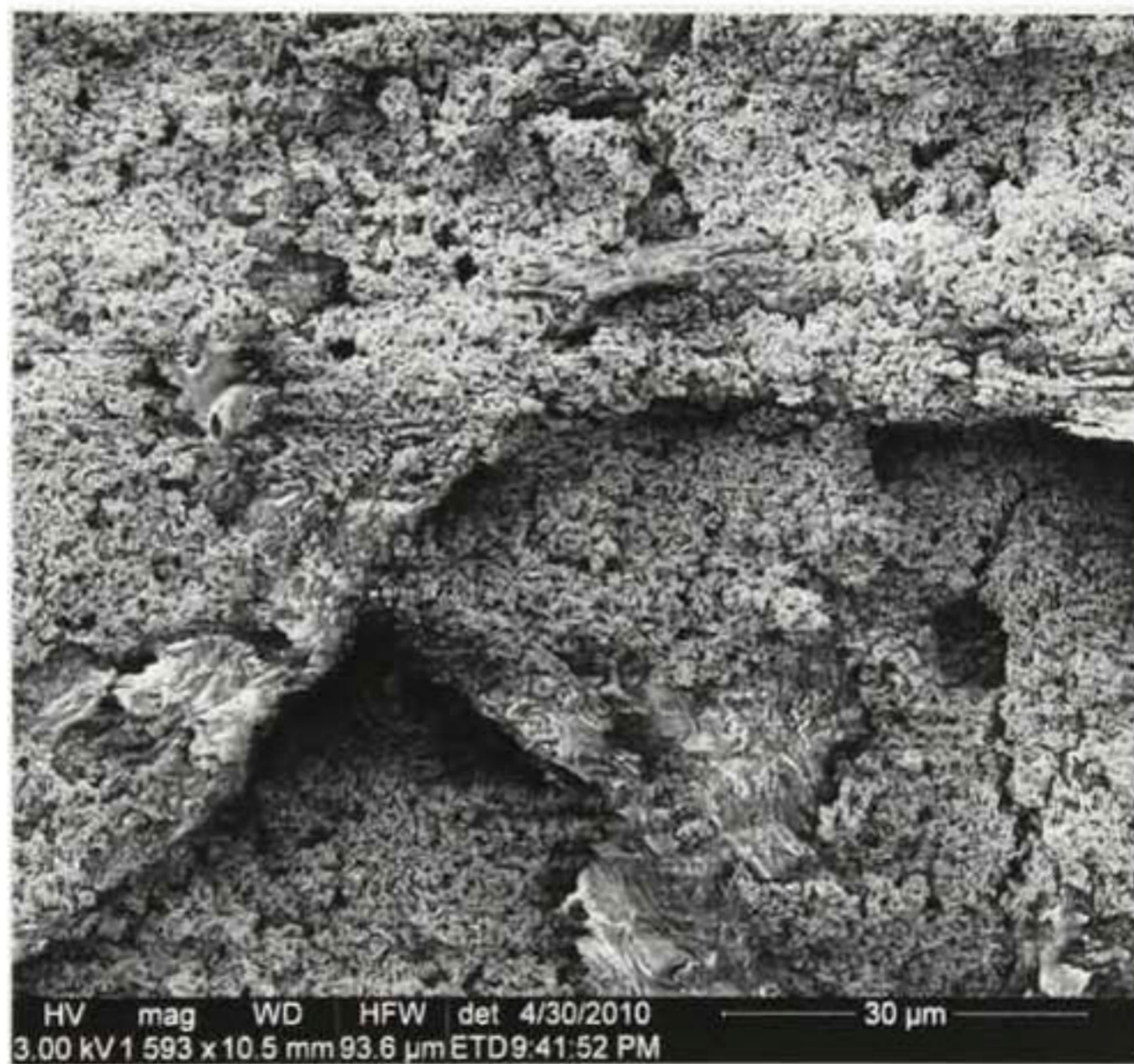
Figure 4. 3 ZnO distributed over the paper surface
