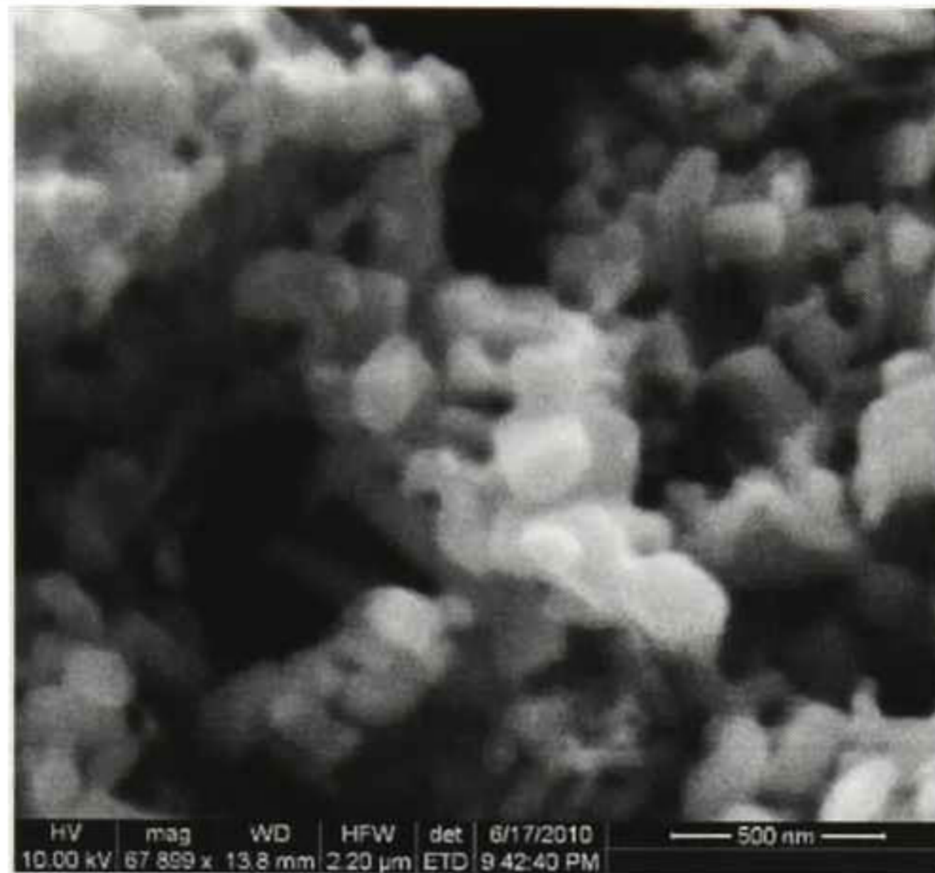
Figure 4. 4 ZnO Crystals agglomerated over the paper surface.
