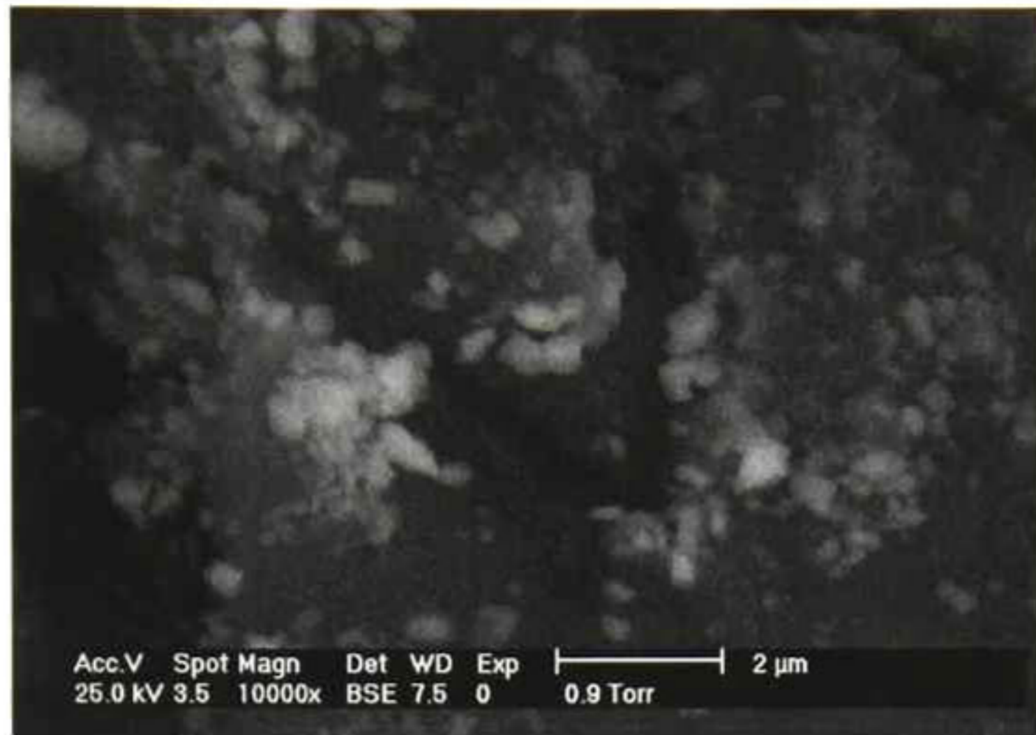
Figure 4. 8 SEM microscopy of a 20-80% ZnO Cellulose pellet cross section.
