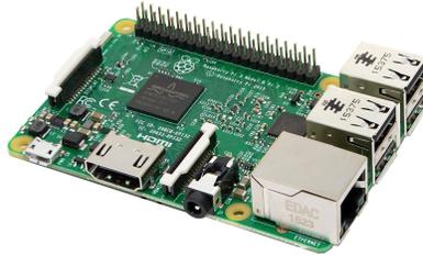
Figura 3.21: *Raspberry Pi 3 Modelo B.*
