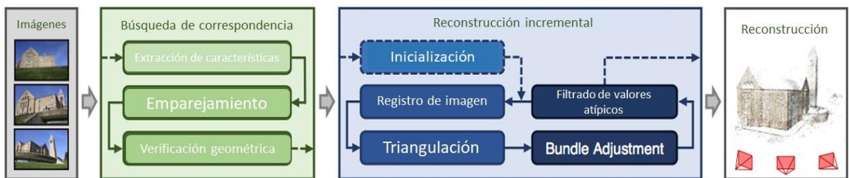
Fig. 4. Pipeline del SfM incremental [13].
