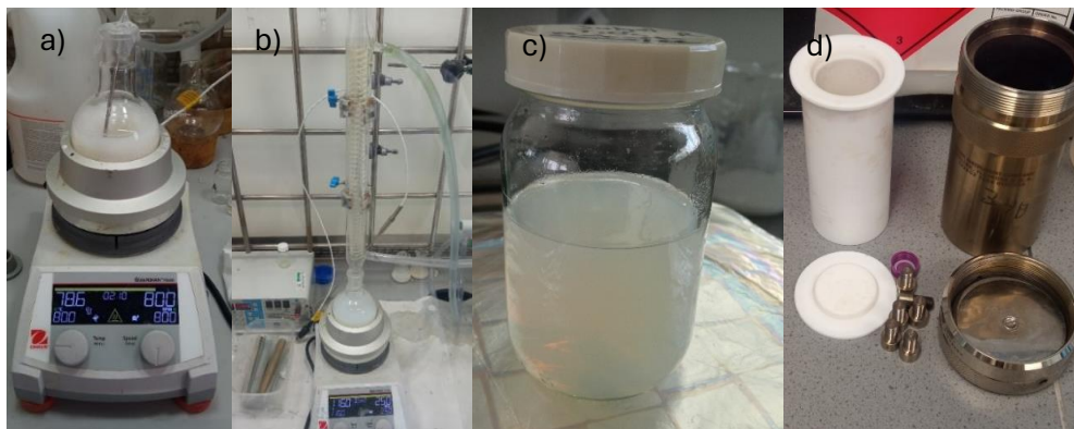
Figure 25. White sol-gel mixture at 80 °C (a) and sol-gel under reflux (b) (step c). Resulting transparent blueish dispersion (d), 200 mL teflon vessel and autoclave digester for hydrothermal treatment (d) (step d).
