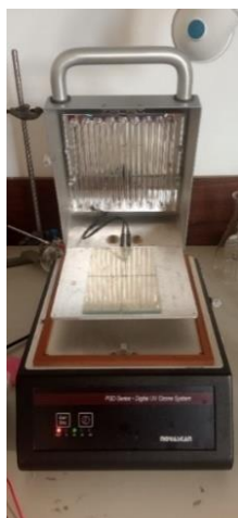
Figure 52. FTOs under 20 min UV- \text{O}_3 treatment.
