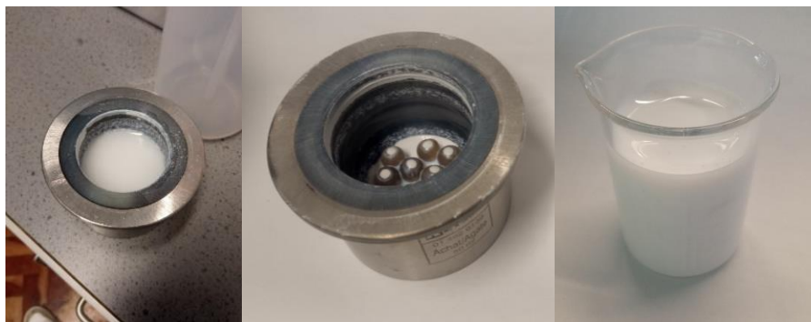
Figure 36. 50 mL agate jar after wet milling (left). Agglomerated \text{TiO}_2 nanoparticles left at the bottom of the jar (center). Stable \text{TiO}_2 anates:rutile (80:20, wt:wt) aqueous solution (right).
