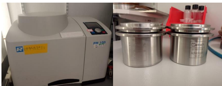
Figure 35. Retsch Planetary Ball Mill PM 100 (left) and 50 mL agate jars used to process paste B (right).
