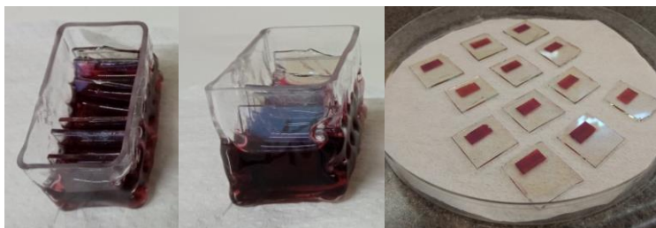
Figure 32. Sensitization of paste A films in D1 dye on ITO-Glass substrates using a glass container (left and center). Dye-sensitized paste A films after 18 hours (right).
