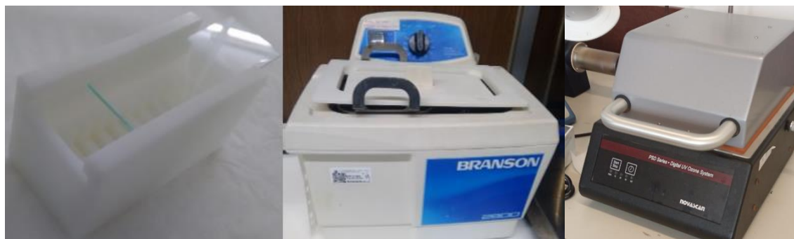
Figure 27. Teflon container for electrode washing (left) and Branson 2800 Ultrasonic Cleaner (center) and Novascan PSD Series Digital UV Ozone System (right) used for the electrode washing.
