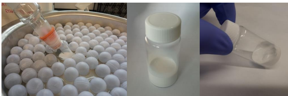
Figure 37. Concentration of \text{TiO}_2 aqueous colloidal solution using a rotary evaporator (left). Viscous paste B (center and right).
