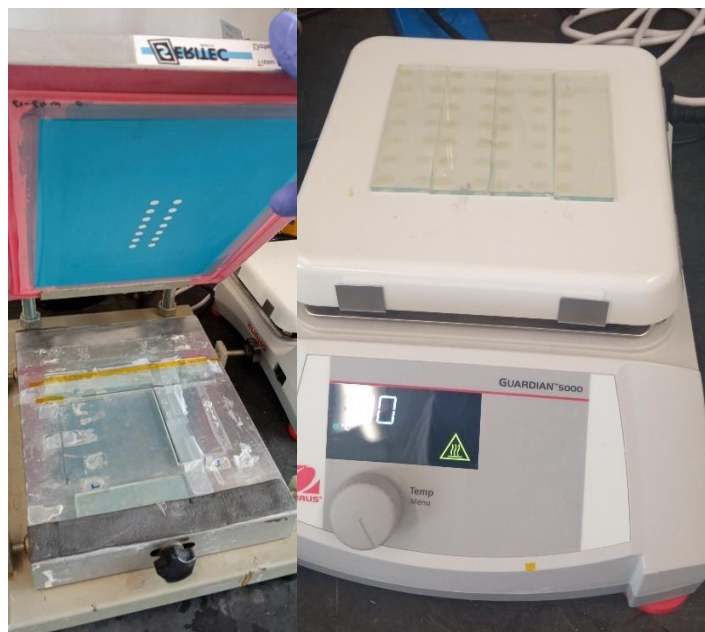
Figure 55. Manual screen-printing for the high-temperature pastes deposition (left) and solvent drying on a hot plate at 120 ^{\circ}\text{C} (right).
