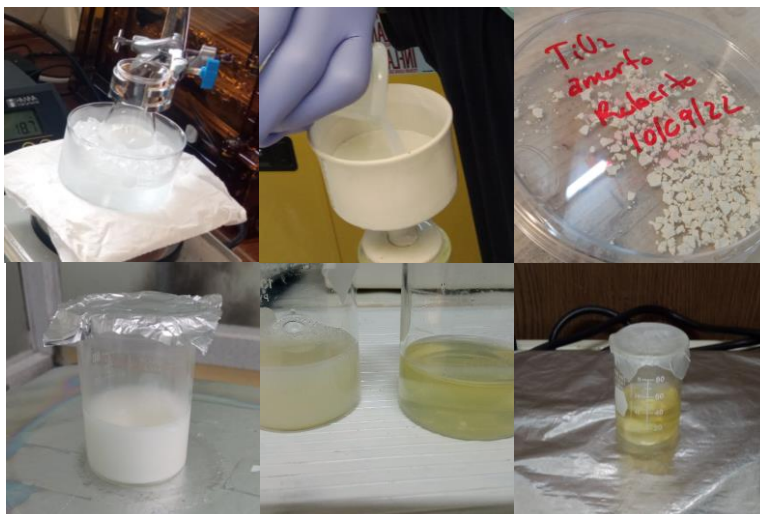
Figure 26. TiO 2 brookite phase synthesis process.
