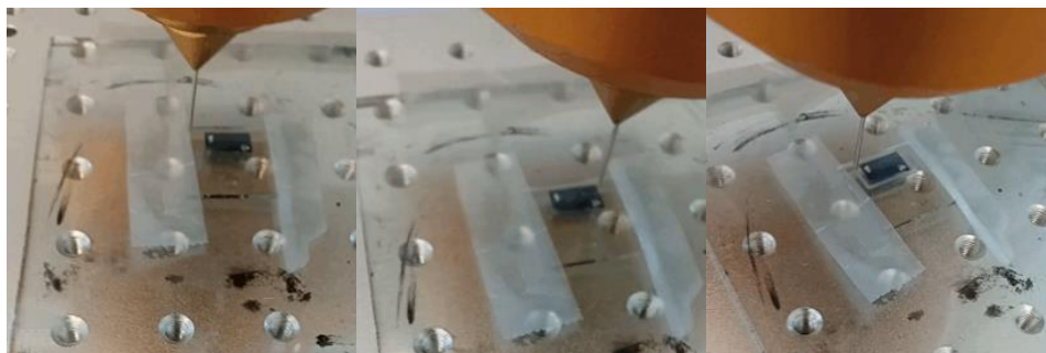
Figure 45. Fixed counter electrode on dispenser plate (left). Glue deposition around the PEDOT film (center and right).
