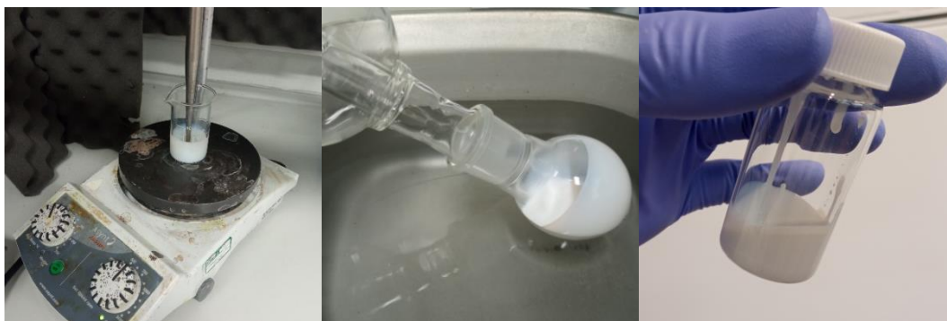
Figure 54. Preparation process of high temperature pastes for DSSC.
