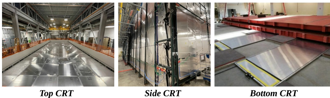
Figure 3.7: ICARUS-T600 CRT system surrounding the detector [5].
