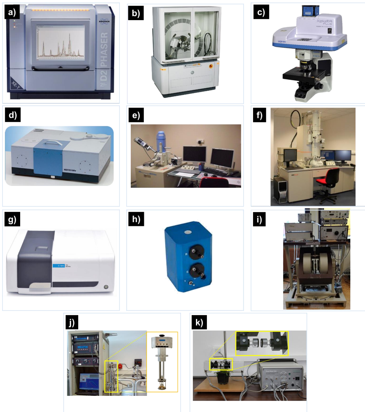
Fig. S.2.1. Equipment used for characterization of the materials manufactured in this research. (a) Bruker D2 PHASER diffractometer, (b) Bragg-Brentano PANalytical Empyrean Bragg-Brentano diffractometer; (c) X'Plora Raman Spectrometer; (d) Vertex 60V Spectrometer ; (e) Scanning Electron Microscope (JEOL, JSM 6510 LV); (f) Microscope JEOL JEM 2100 HR -IMMM; (g) UV-Vis Spectrophotometer, Agilent Cary ; (h) Ocean Optics ISP-REF integrating sphere; (i) Electron paramagnetic resonance spectrometer; (j) Novocontrol Broadband Dielectric Spectrometer (Alpha-A High-Performance Frequency Analyzer); (k) Dual-beam spectrophotometer (Perkin Elmer) with Dual PAM-100.
