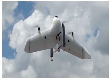
Figura 1.7: Transition Optimization for a VTOL Tail-Sitter UAV [4].
