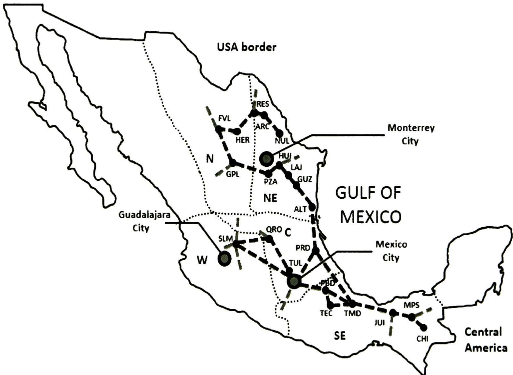
Fig. 5.1. Simplified geographical representation of the MIS showing the location of major generators and transmission paths.
