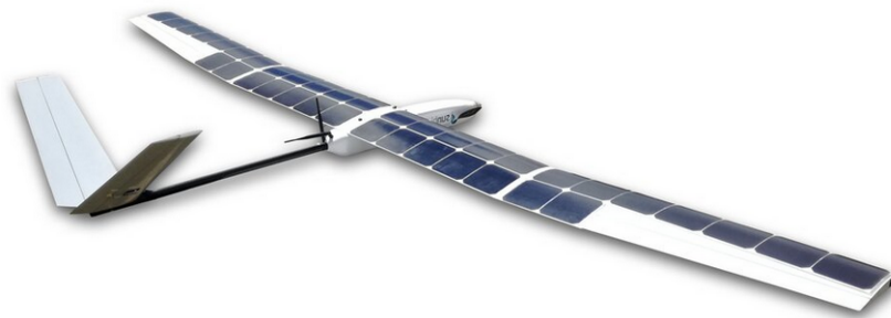
Figura 1.1: UAV solar SB4 Phoenix [9].
