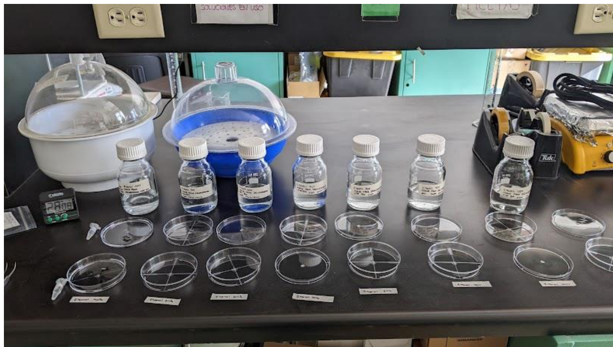
Figure 2.5 Photograph showing samples of bioanodes submitted to dehydration in ethanol solutions.
