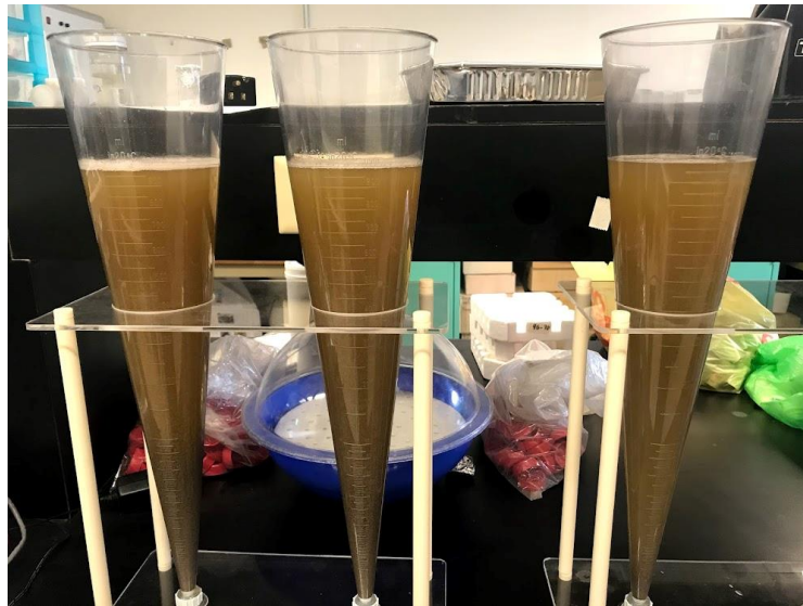
Figure 2.8 Imhoff cones with PWW for the measurement of settleable solids.
